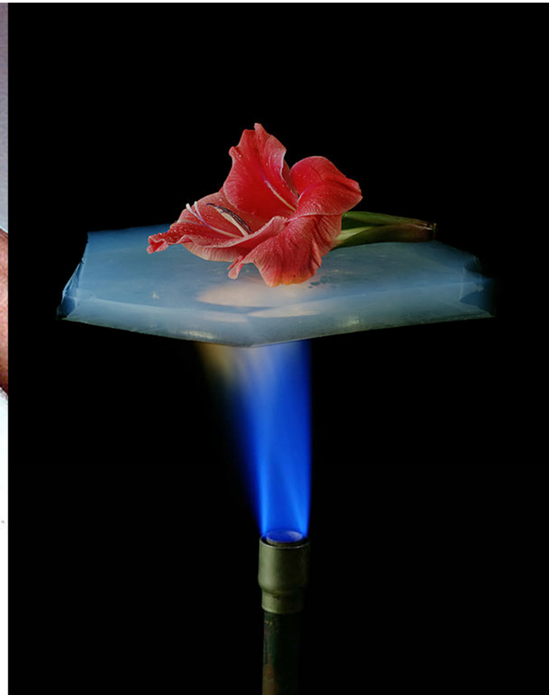
A flower is on a piece of aerogel which is suspended over a flame from a Bunsen burner. Aerogel has excellent insulating properties, and the flower is protected from the flame. – Image: Aerogelflower filtered
